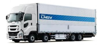
Isuzu GIGA LNG Vehicle: Specifications: GVW 25 ton, 243kW, 9 gears (Automatic AMT)
