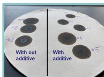
Figure 43 Blend stability test results for CFP-based bio-oil and HTL-based bio-crude.
