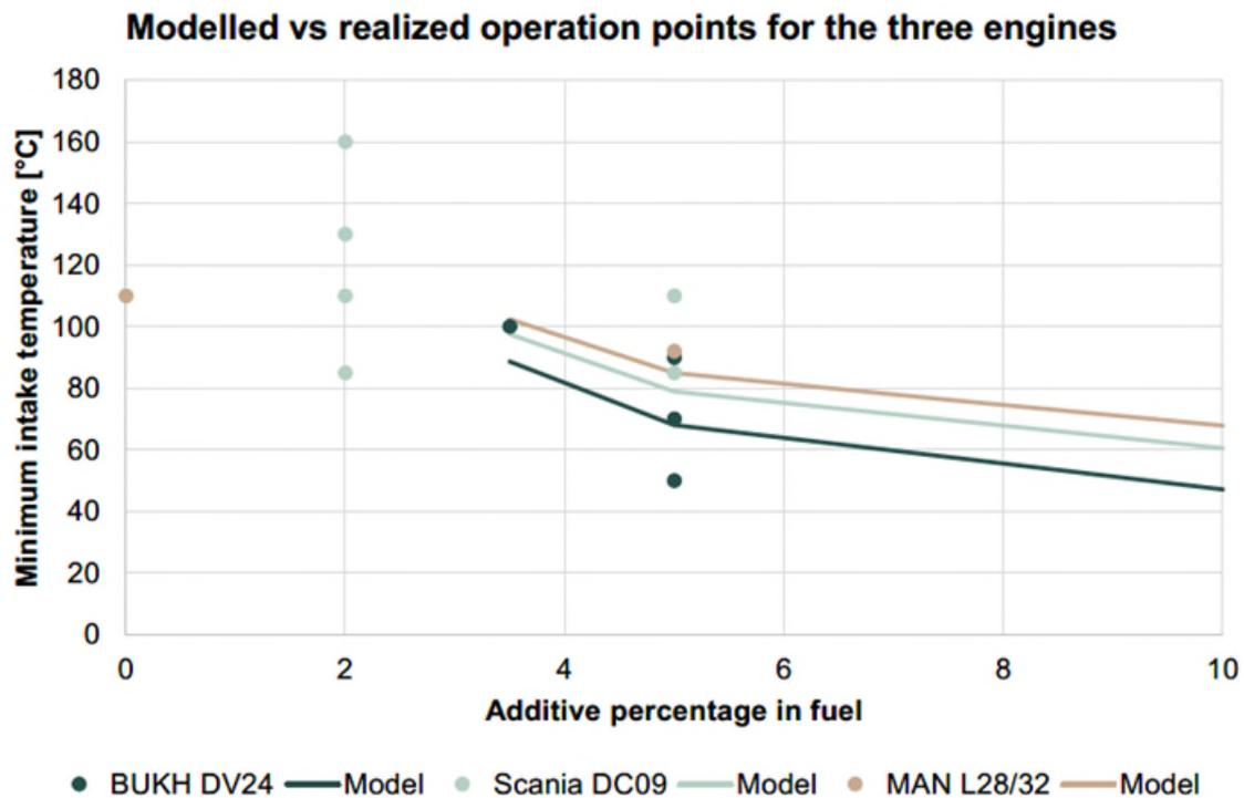
Figure 59 Test data from experimental methanol engines in Denmark
