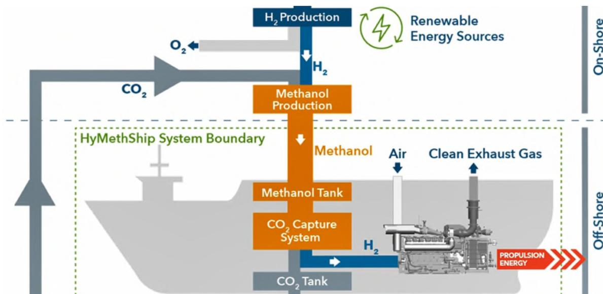
Figure 41 Pre-combustion CO<sub>2</sub>-capture concept for methanol ship (LEC)
