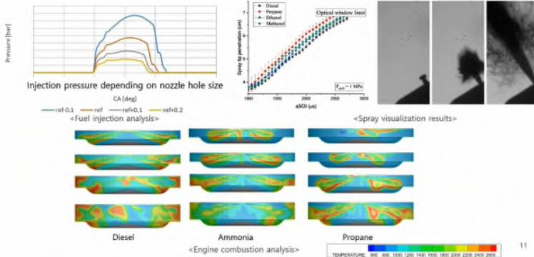
Figure 15 Injection and ignition processes with some advanced marine fuels
