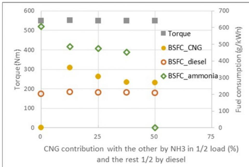
Figure 6 Torque output and brake specific fuel consumption with ammonia-CNG-diesel triple fuel combustion at full load condition.
