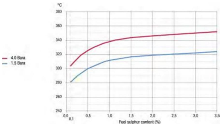
Figure 28: Minimum SCR operating temperature as function of fuel sulfur content. Curves for high-pressure (red) and low-pressure (blue) SCR installations. MAN 2-stroke Emission Project Guide, 2022 (12.th edition)
