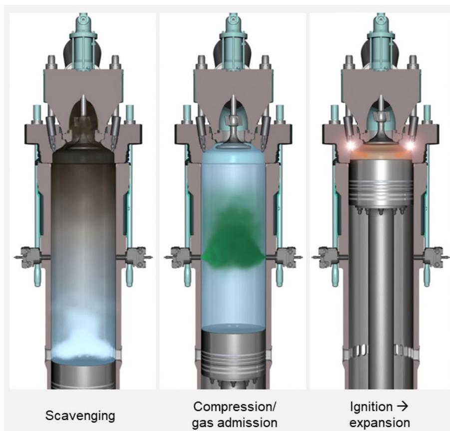
Figure 3 Illustration of WinGD's X-DF working principle (Nylund, 2013)
