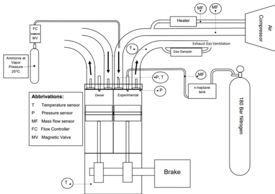
Figure 64 DTU Test engine set-up.
