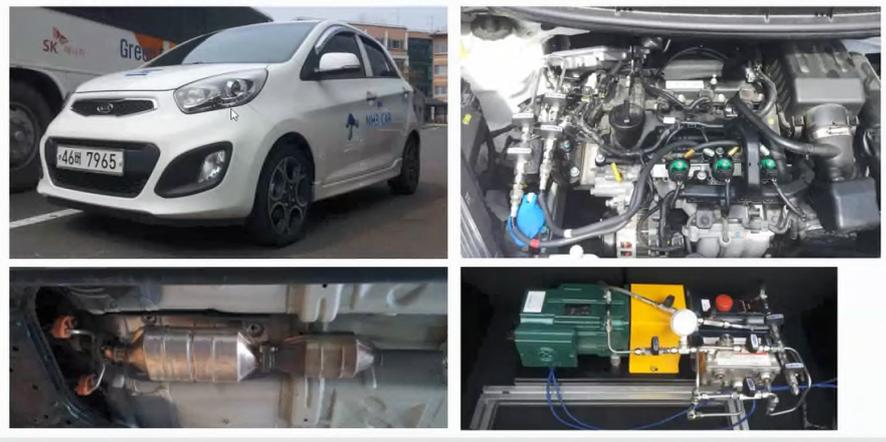
Figure 79 A working dual fuel ammonia-gasoline vehicle.
