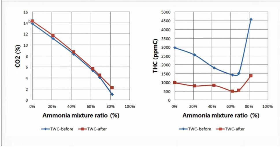
Figure 77 Mixtures above 60% ammonia lead to higher unburnt hydrocarbon emissions.
