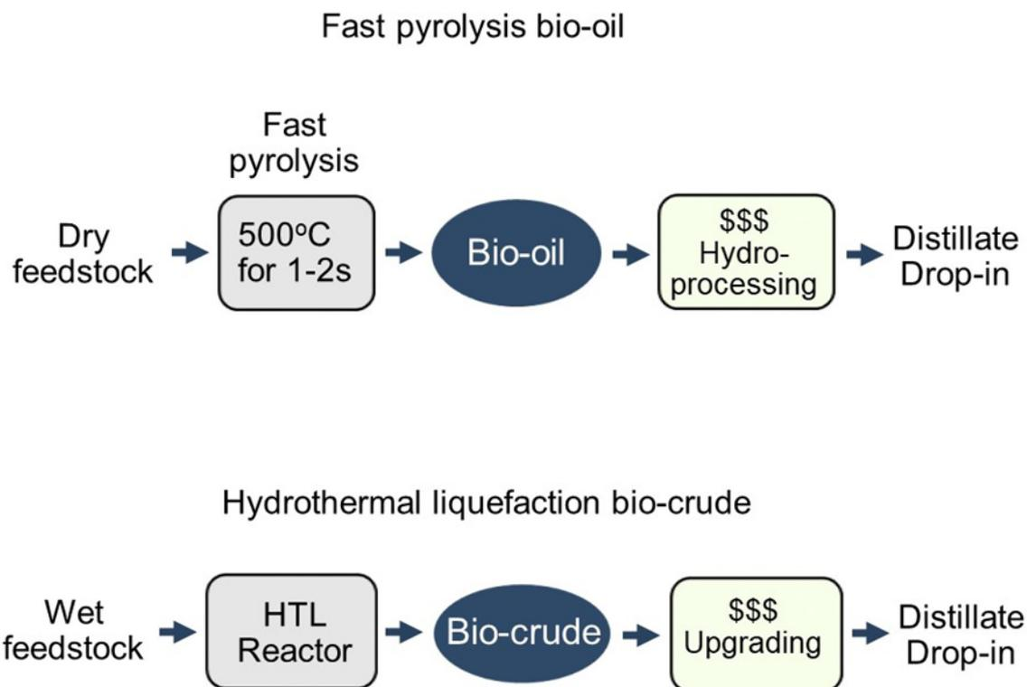
*Figure 42 Bio-intermediate production schematic via fast pyrolysis and hydrothermal liquefaction.*
