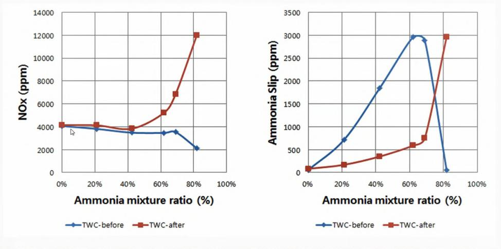
Figure 78 Mixtures above 60% ammonia lead to higher NOx and ammonia emissions.
