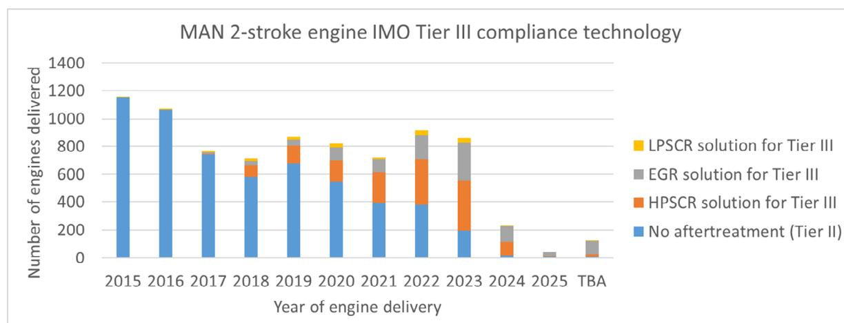
Figure 24: Technology choice for IMO Tier III compliance
