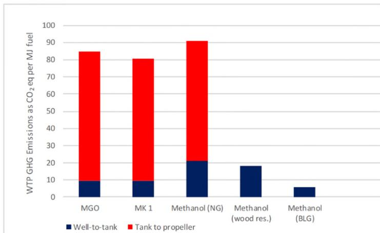
Figure 60 GHG emissions per MJ fuel for methanol from natural, wood residues, and black liquor gasification (BLG) as compared to marine gasoil and MK 1 diesel. (Ellis *et al.*, 2018).
