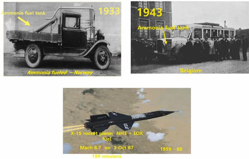
Figure 71 Ammonia was used as fuel for trucks, buses and rocket planes in the past.
