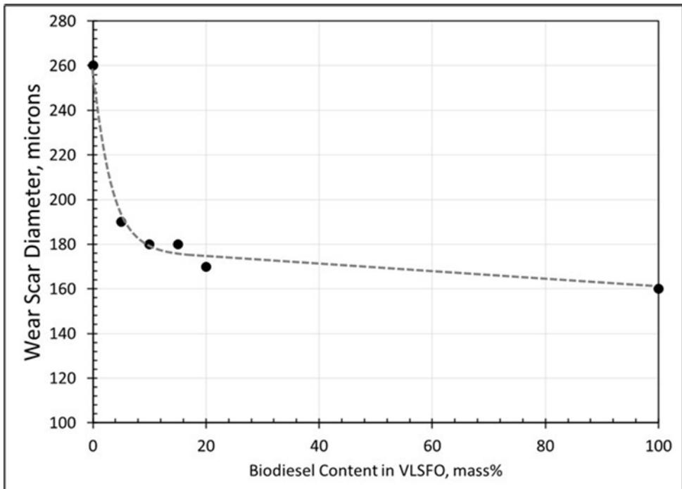
Figure 47 Wear scar diameter measurements for biodiesel blends with VLSFO. Results show a significant reduction in wear scar diameter (improved lubricity) with added biodiesel.
