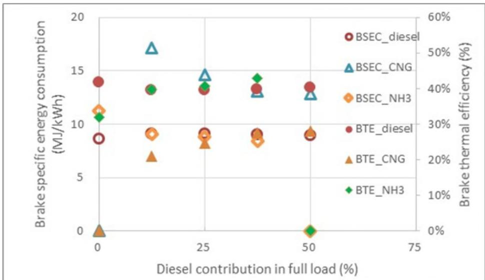
Figure 8 Brake specific energy consumptions and thermal efficiencies from ammonia-CNG-diesel triple fuel combustion at full load condition.
