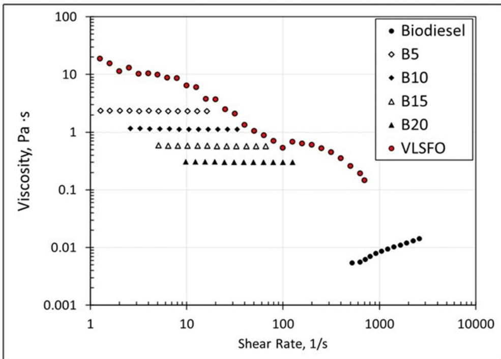
Figure 48 Dynamic viscosity of VLSFO with biodiesel additions up to 20%.
