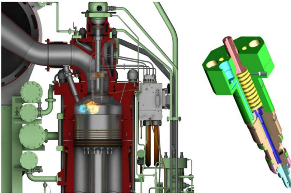
Figure 2 Illustration of the ME-GI working principle (left) and gas injector design (right) as key system feature (Juliussen)
