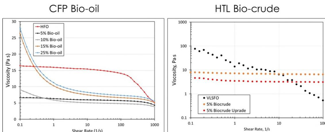
Figure 44 Viscosity versus shear rate for blends of bio-oil and bio-crude with VLSFO at 25°C.
