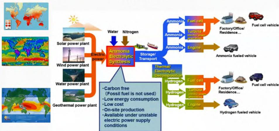
Figure 69 Ammonia can serve directly as a fuel or as a hydrogen carrier.
