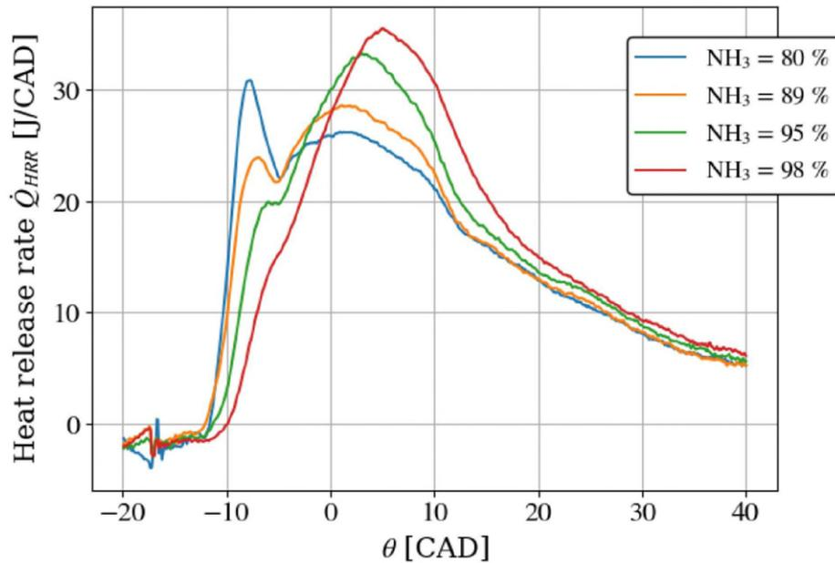
Figure 65 Heat release rates for increasing ammonia energy, with a constant  $\lambda = 1.1$
