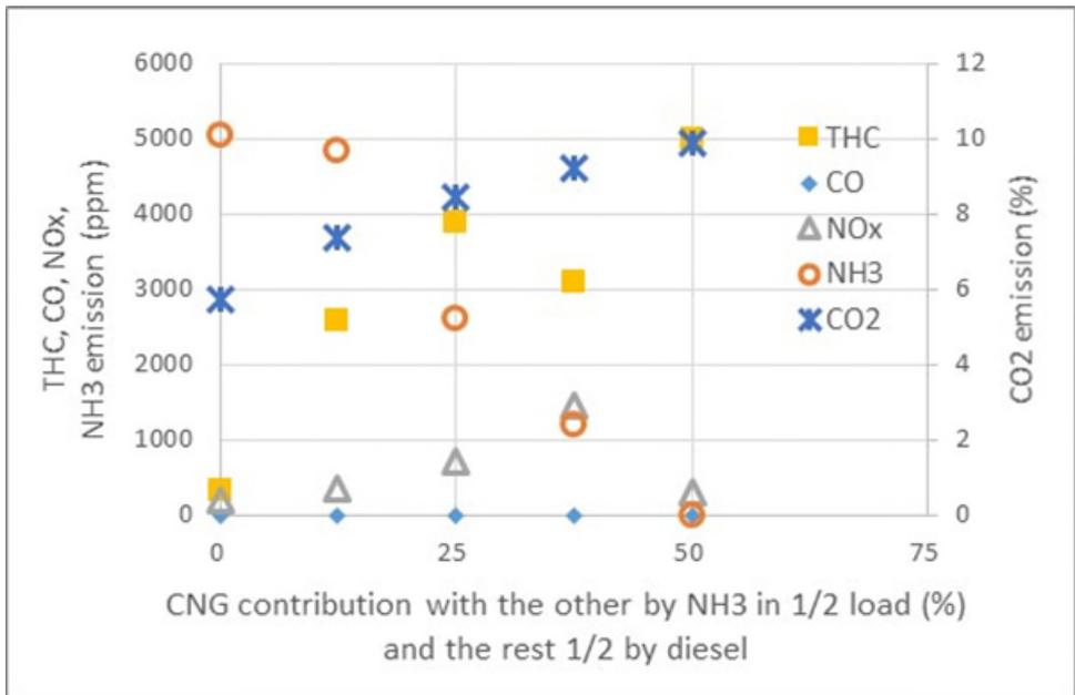
Figure 7 Emissions from ammonia-CNG-diesel triple fuel combustion at full load condition
