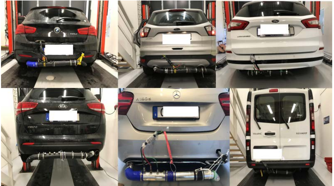
Figure 39. Example of installation of the sensors during tests with the Mini-PEMS system.
