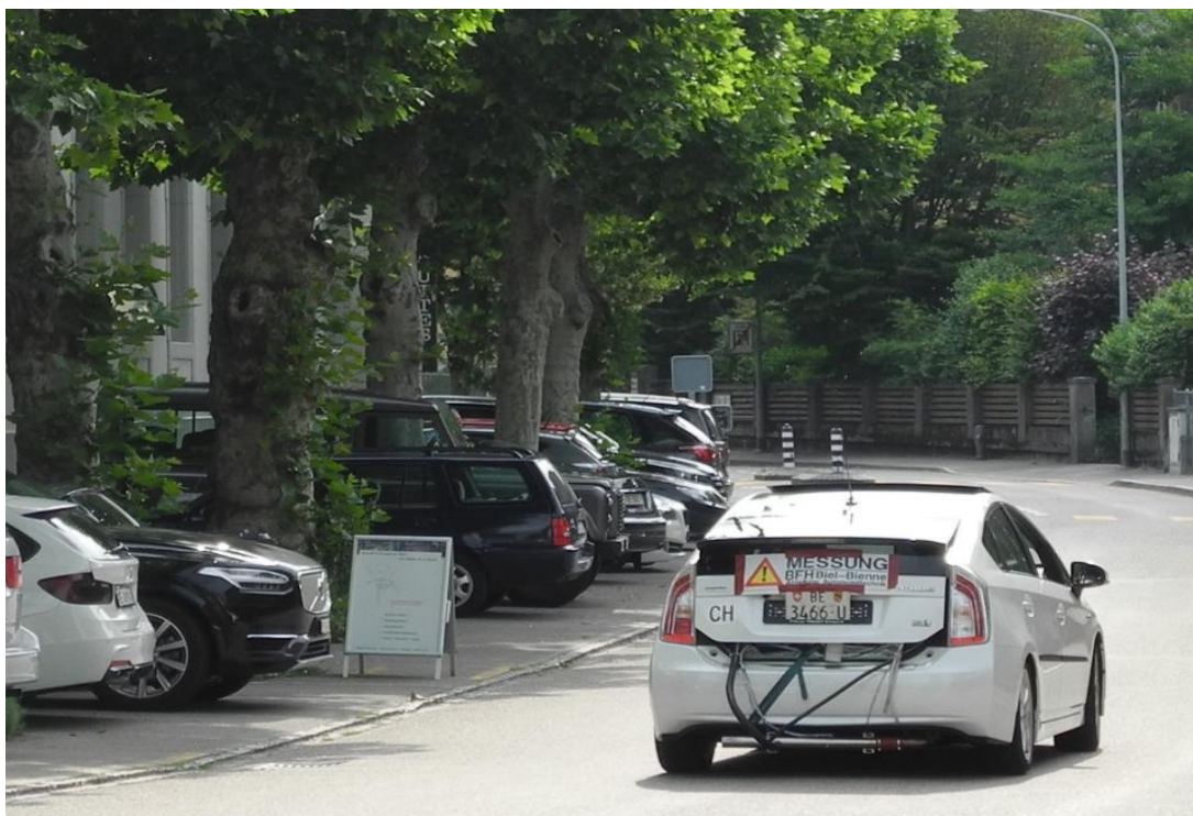
Test vehicle on the road equipped with PEMS
