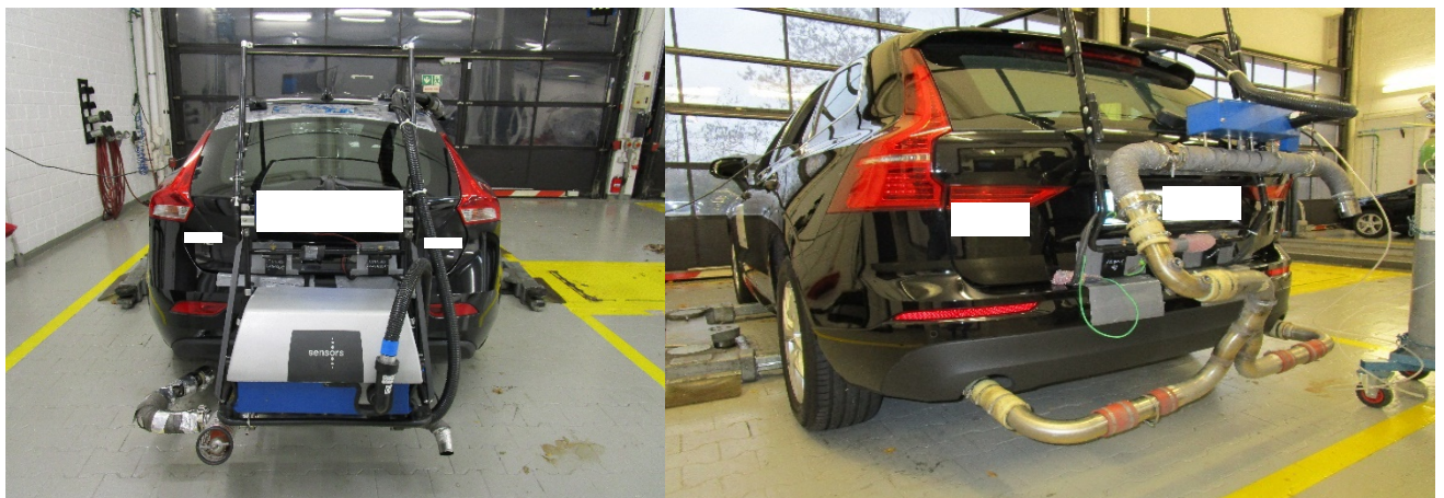
Figure 29. Example of PEMS-installations. Mini-PEMS and Full-PEMS are measured in parallel
