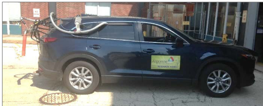
Figure 7: Mazda CX-9 Test Vehicle with RDE Equipment Installed
