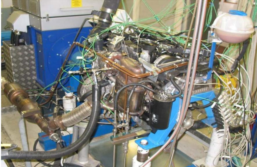
*Figure 8: Test engine with exhaust after treatment components and test bench brake*
