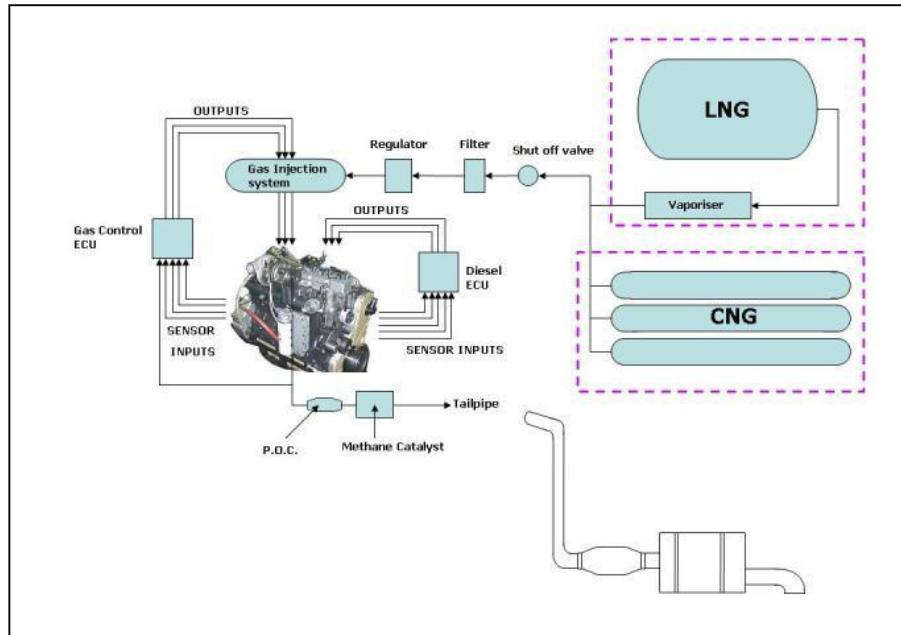
**Figure 8.** Hardstaff OIGI Diesel dual fuel system
