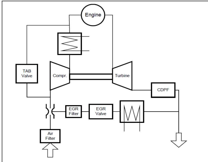
**Figure 6.** Basic lay-out of PACCOLD-EGR system
