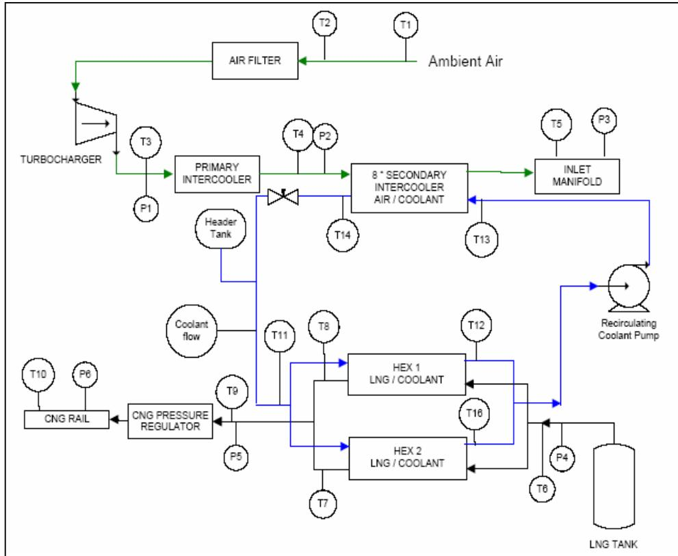
**Figure 7.** Basic lay-out of SIC system with parallel HEX arrangement
