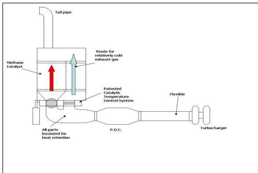
**Figure 9.** Hardstaff patented catalytic temperature control
