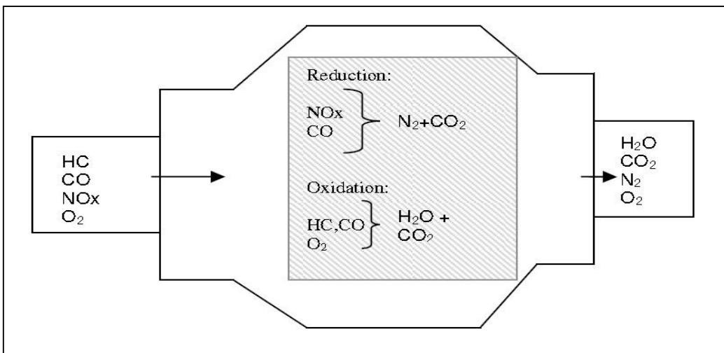
**Figure 2.** Chemical processes in a three way catalyst [1]
