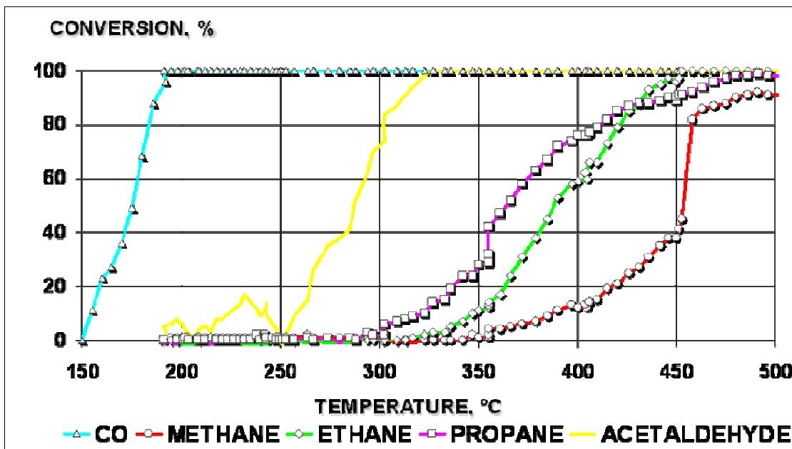
Figure 3. Conversion rate vs. exhaust temperature (Source: Kemira)
