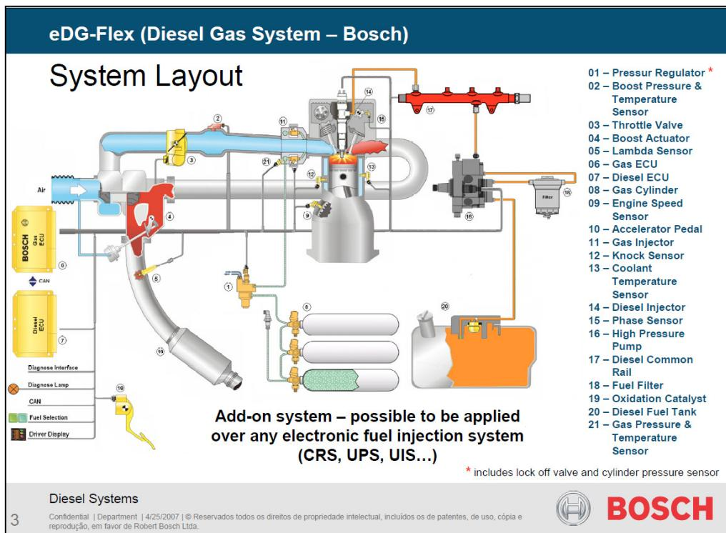
Figure 10. Bosch Dual Fuel system eDG-Flex (Source: Bosch Brazil)
