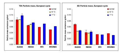
Figure 41. Particle mass emissions with TDI and IDI cars.
