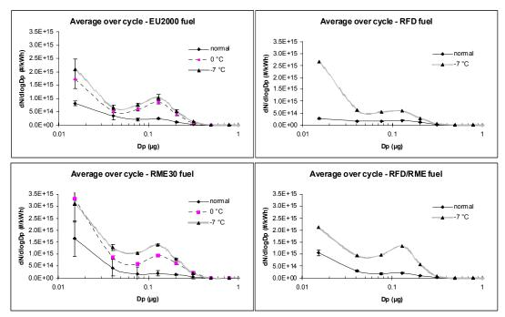
Figure 21. Particle number distributions over the 16-minute cycle, medium-duty engine.
