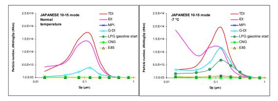
Figure 49. Particle number size distributions over the Japanese 10-15 mode test cycle.
