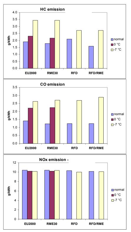
Figure 11. Regulated gaseous emissions, medium-duty engine.
