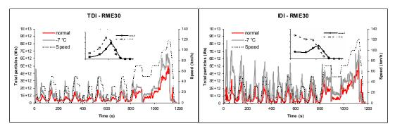
*Figure 44. Particle flow and number distribution over the European test cycle using RME30 fuel, diesel cars.*
