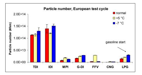
*Figure 34. Total particle number emissions over the European test cycle at different temperatures, light-duty cars.*
