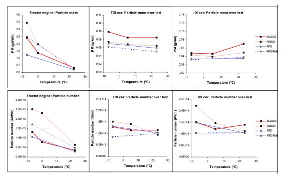
*Figure 45. Summary of particle mass and number results with tractor engine and diesel cars.*
