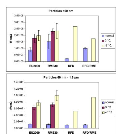
Figure 20. Number concentration of particles in two size classes, medium-duty engine.
