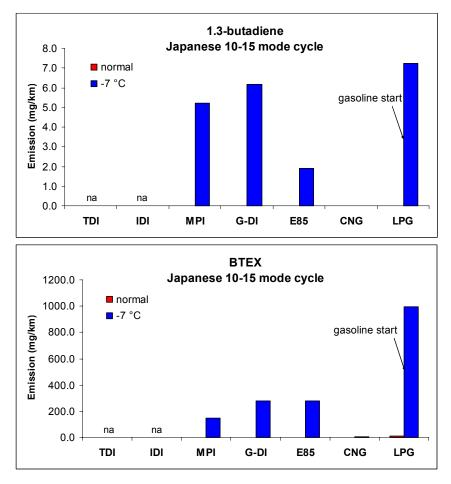
*Figure 46. 1,3-butadiene and sum of benzene, toluene, ethylbenzene and xylenes over the Japanese 10-15 mode test cycle.*
