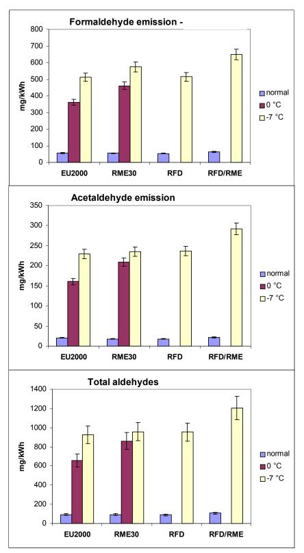
Figure 12. Aldehyde emissions with the medium-duty engine.
