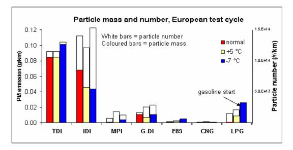
*Figure 50. Overall summary of particle mass and number emissions with light-duty cars.*
