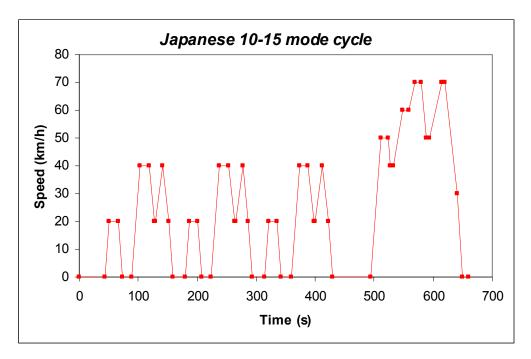
Figure 2. Japanese 10-15 mode test cycle.
