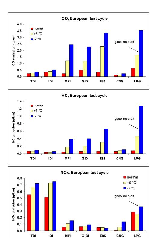
Figure 24. Regulated gaseous emissions over the European test cycle, light-duty cars.
