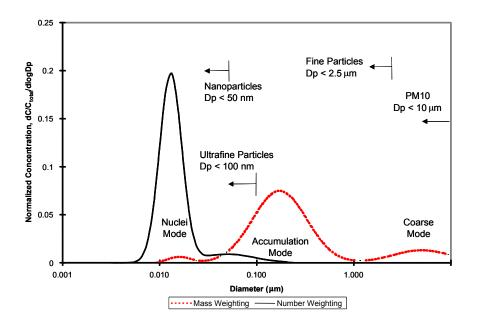
Figure 3. Schematic Figure of number and mass size distribution with both nucleation and accumulation mode, diesel exhaust gas [5].
