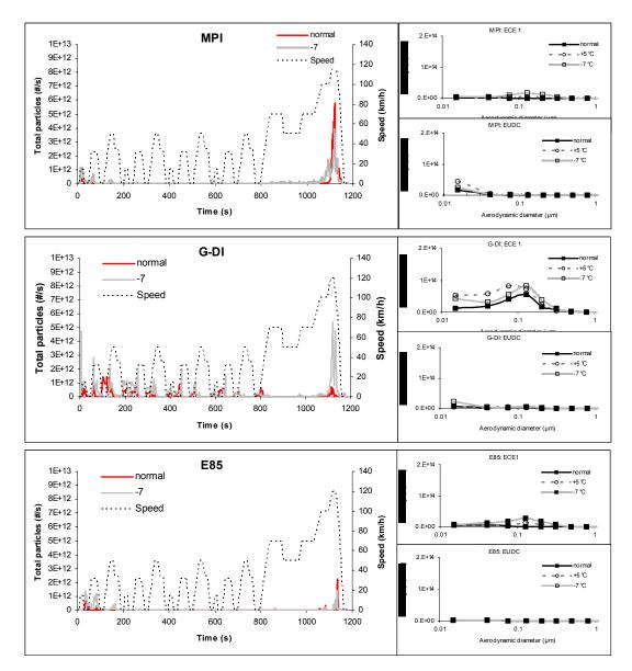
*Figure 36. Particle number flow over the European test cycle with MPI, G-DI and E85 (FFV) cars.*
