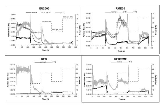
Figure 19. Particle number flow, medium-duty engine.
