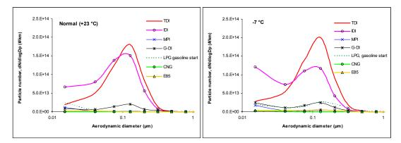
Figure 33. Particle number size distributions over the European test cycle at +23 °C and -7 °C temperatures, light-duty cars.
