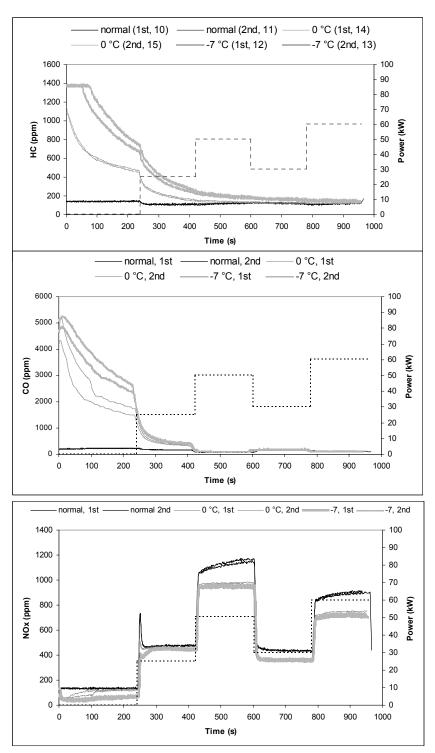
*Figure 10. CO, HC and NO<sub>x</sub> concentrations, medium-duty engine.*
