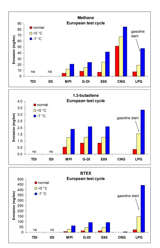
*Figure 27. Methane, 1,3-butadiene and sum of benzene, toluene, ethylbenzene and xylenes over the European test cycle, light-duty cars.*
