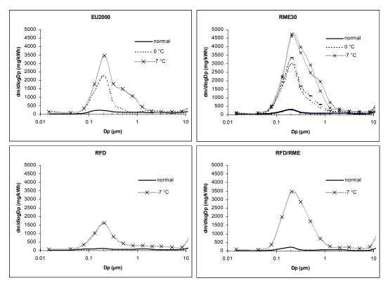
Figure 15. Particle mass distribution results, medium-duty engine.
