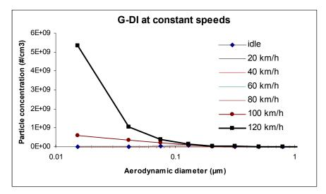
*Figure 38. Particle number size distribution at constant speeds with G-DI car at normal temperature.*
