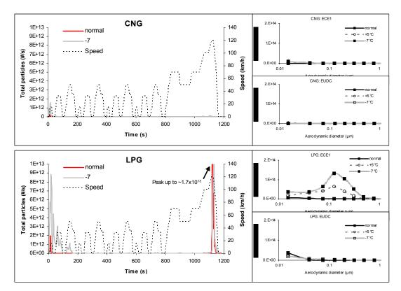
Figure 37. Particle number flow over the European test cycle with the CNG and LPG cars.
