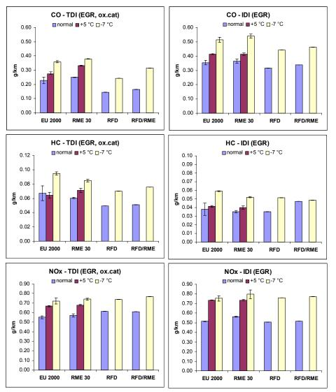
Figure 39. CO, HC and  $NO_x$  emissions over the European test cycle with the TDI and IDI cars.
