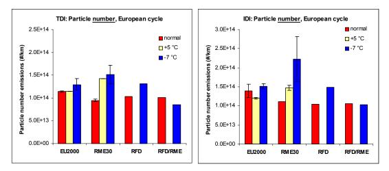
Figure 43. Total number of particles over the European test cycle, TDI and IDI cars.
