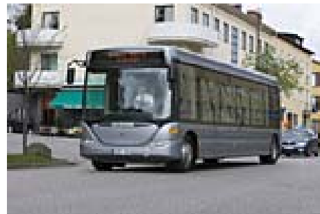
Scania's ethanol hybrid bus ( www.scania.com ).
