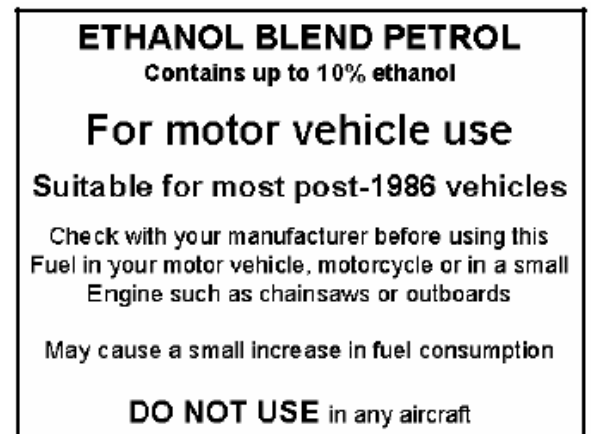
The Australian label for ethanol blended gasoline. Source: Egebäck et al. MTC report 5407.
