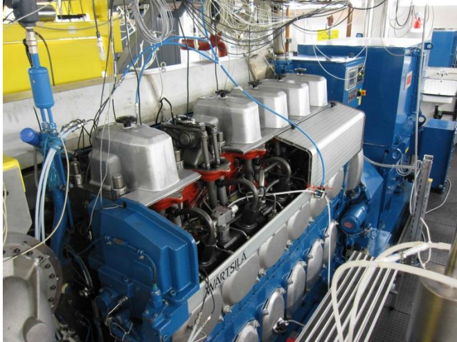
Fig. 7 Large Engine Research Facility at Paul Scherrer Institute (PSI) in Switzerland with a Test Rig for a 1.2-MW Mechanical Output Diesel Engine
