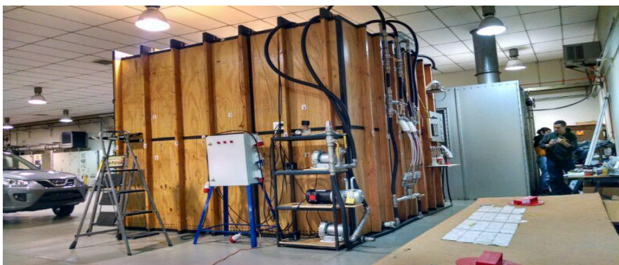
Fig. 1 Chamber for Photochemical Aging of Vehicle Primary Emission
