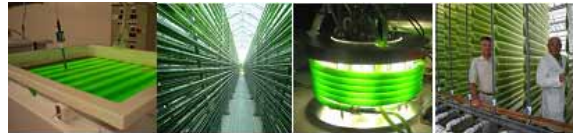
Figure 4 Various designs of PBRs used in industry. From left to right: Brite Box PBR (Source: Natural Resources Canada); Tubular PBR (Image Source: Bioprodukte Prof. Steinberg); Wrapped PBR (Source: The University of Georgia); High Density Vertical Bioreactor (Source: Vertigro Products, Inc.).
